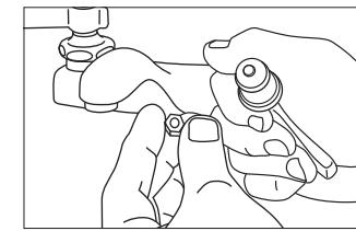
STEP 5 - Reassemble sleeve (D) on lightly lubricated stem (C). With new parts add seat (F) O-Ring (G) seat washer (H) retainer (I) and washer (J) on stem (C) and screw nut tightly on stem.
