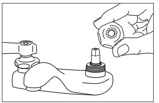
STEP 6 - Reposition washer and O-Ring (B) on stem (C) add to sleeve (D). Replace cartridge in the direction of closing until the cartridge is in the desired position for convenient operation. Remove handle. Lock cartridge in place by securely tightening Cap Nut (A) to 20 - 27 ft. lbs torque.
