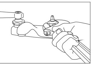
STEP 7 - Replace Cap Nut (A) and partially tighten. Replace handle and rotate cartridge in the direction of closing until the cartridge is in the desired position for convenient operation. Remove handle. Lock cartridge in place by securely tightening Cap Nut (A) to 20 - 27 ft. lbs torque.
