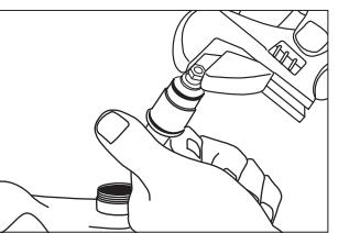
STEP 3 - Unscrew stem nut (K) at the bottom of the cartridge with a flat wrench using a handle as lever to assist removal.
