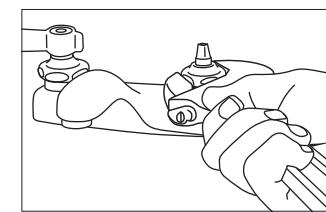
STEP 1 - Turn off water at stop or main valve. Remove handle assembly and with flat face wrench, remove cap nut (A).
