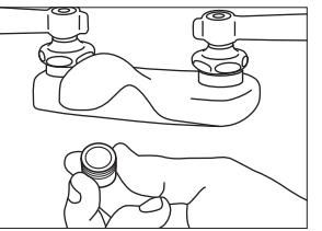
STEP 8 - Turn water on at main valve or stop. Remove aerator. Turn faucet on to "full" allowing sediment to flush from lines and replace aerator cartridge.
