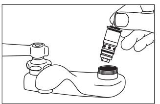
STEP 2 - Remove cartridge from faucet. Flush out any rust or chips that may be in body. DO NOT use file or abrasives to clean out body.
