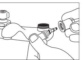
STEP 4 - Turn sleeve (D) off stem (C) by holding handle and turn sleeve by hand. As sleeve is removed from stem, seat (F) O-Ring (G) seat washer (H) retainer (I) and washer (J) will be forced off the stem.
